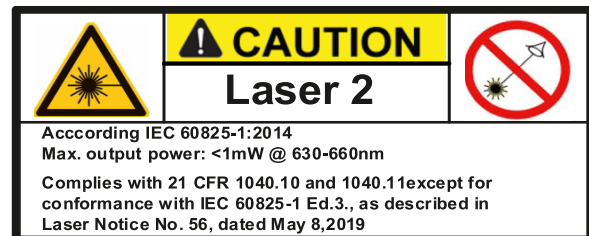
Figure 2: Product labeling "Class 2 laser"
