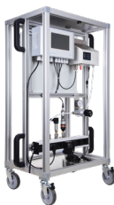
Compressed air quality measurement
