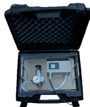
Compressed air quality measurement
