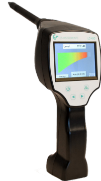
LD 450 with focus tube and focus tip for exact detection.
