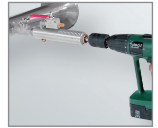
Drill under pressure with the CS drilling jig
