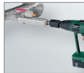
Drill under pressure with the CS drilling jig
